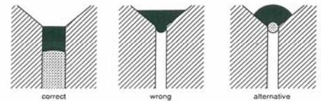
In corner joints too, the insertion of a release tape or backer rod is required, otherwise the sealant will fail during expansion of the joint.
